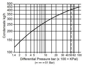
Note: Minimum Differential pressure for satisfactory operation 1.4 bar g with Positive Pressure and Discharge to atmosphere.
